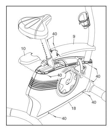
Remove the five M4 x 16mm Screws (40) from the Right Shield (18). Then, gently move the Right Shield away from the frame.
